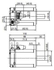
① Encoder connector 2 Motor connector
